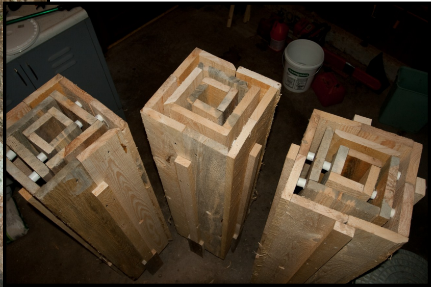
Interior: a modified stacking rocket box design was constructed from rough-sawn pine on a cedar base
